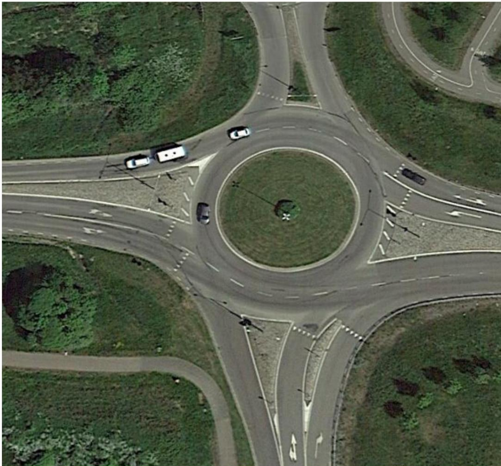
Example of a typical multi-lane roundabout where one or more lanes only lead to the exit (two lanes lead to the east exit and one to the west). This particular roundabout is relatively newly built and is on a state road.
