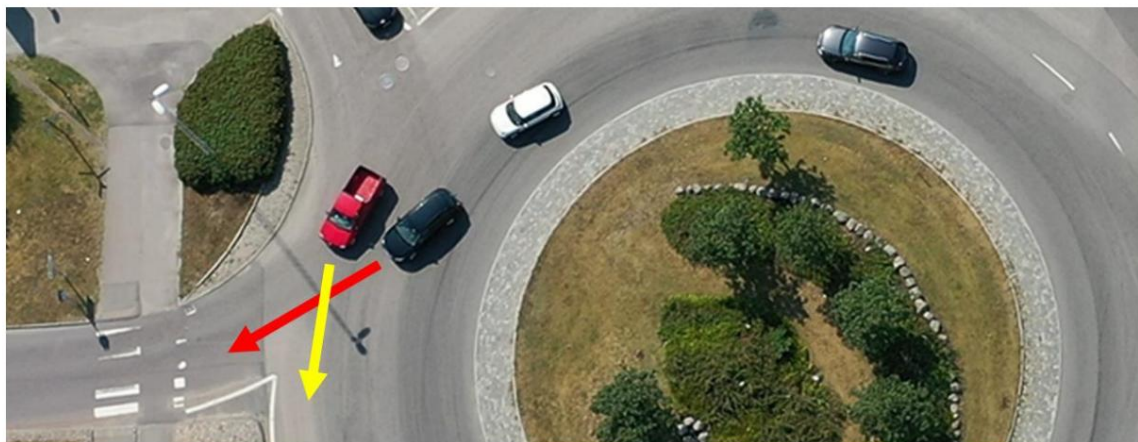
WSP's drone filming, example of conflict in today's design of multi-lane circulation site. The black car must panic brake to a complete stop for the red car.
