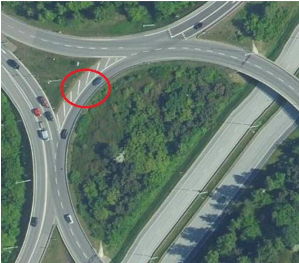
Example 3: Two fields are not always used in practice with today's design, which is why painting has sometimes taken place. In this type of location, there is potential in using the two existing fields with a different design, which can increase accessibility.
