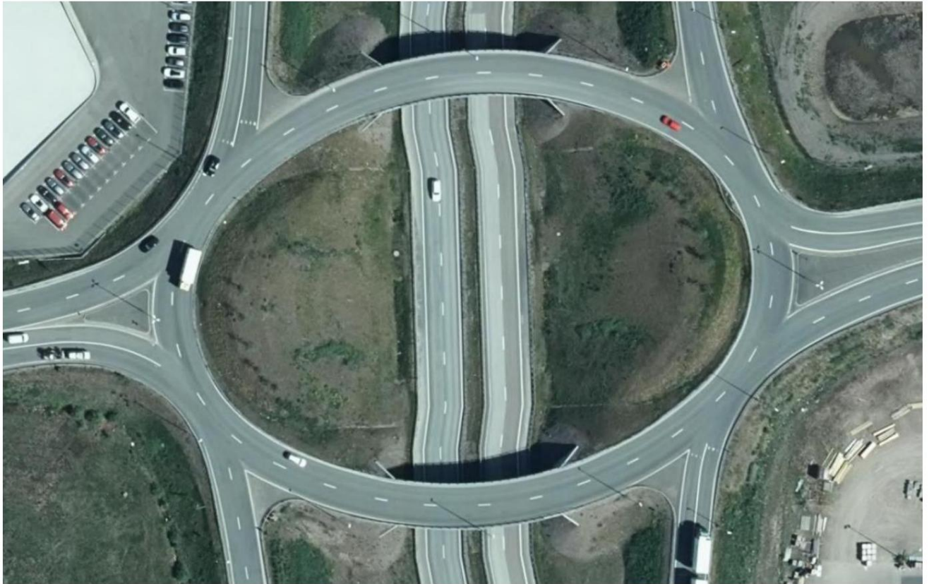
Example of an oval roundabout, where the radius changes inside the roundabout, Tpl Rebbelberga in Ängelholm.
