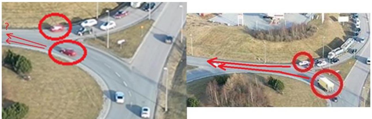
Example 1: A car turning right also gives way to vehicles that are in the inner lane. Actually, they could have run parallel, whereupon the passability could potentially have increased, as there are two lanes towards the exit in this case.
