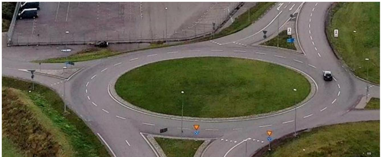
Example of drone footage (performed by WSP) over typical multi-lane roundabout where both lanes are painted all the way around (ie is like Example 1 above).
