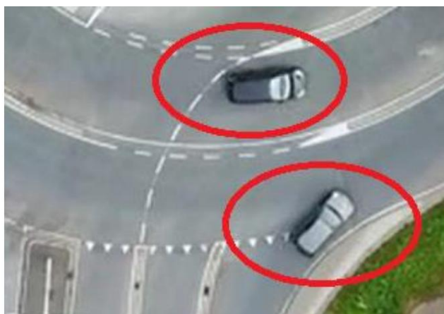
A drone footage of a Turbo roundabout shows that the drivers understand that in practice you don't always have to give way to the inner roundabout. The same is also seen in the Munkebäcksmotet in Gothenburg, where one of the entrances has a design that partially resembles a Hassel circle where you don't always have to give way for the inner field (see further in later chapters where comparisons with the Munkebäcksmotet are made).
